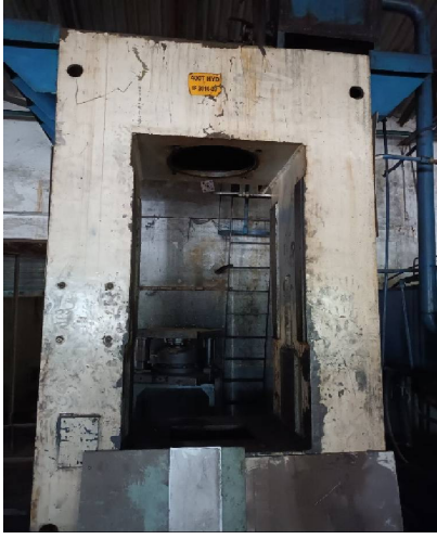
400 Ton, Hydraulic Press, Frame Table size: 560 x 560 mm Not Operational
